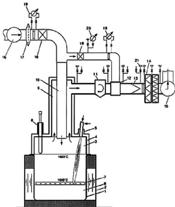
1 – ceramic crucible; 2 – melting assembly; 3 – incineration area; 4 – sodium cooled steel lid of the melting assembly; 5 – gas burner to increase the temperature of the gas phase; 6 – MRW; 7 – slag; 8 – pyrometer in a ceramic shell; 9 – mixer chamber; 10 – ceramic tube of the mixer chamber; 11 – precipitator; 12 – mixer chamber; 13 – sock filter; 14 – aerosol filter; 15 – gas blower; 16 – air blower; 17 – filter; 18 – valve; 19 – flowmeter; 20 – compound gauge; 21 – analytical filter
